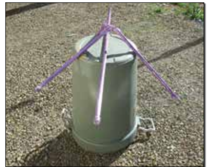
To get paint to stick to PVC pipe, first coat the pipe with “purple plague” PVC primer, the stuff you usually use on PVC joints before glueing.
