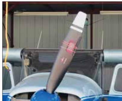
Strap an iPhone to the propeller to time the mags using iHandy Carpenter , a $1.99 iPhone app from the iTunes app store.
