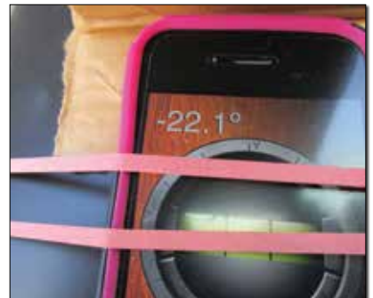
Compared to expensive instruments in a college physics department, the iPhone app was easily within a tenth of a degree accuracy.
