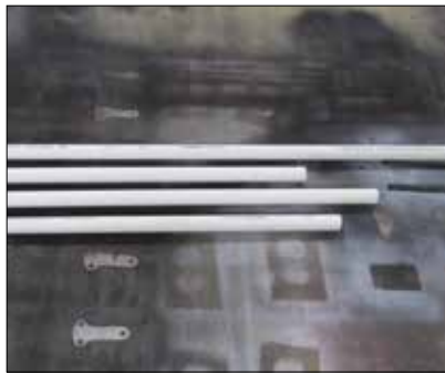
Even paint that is supposed to be good for plastics typically won't stick to PVC water pipe.
