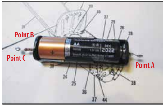
Measure volts from point A to point B. Attach a 1.0k ohm resistor to the positive end of the battery and measure current from point A to point C. Read the resistance of the resistor from point B to point C.
