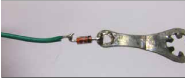
(Above) A diode temperature sensor mounted to a #4 solder lug for heat transfer. (Right) The fan mounted to the rear of the transponder case with the diode temperature sensor bolted to the right. Note the heat shrink on the diode.
