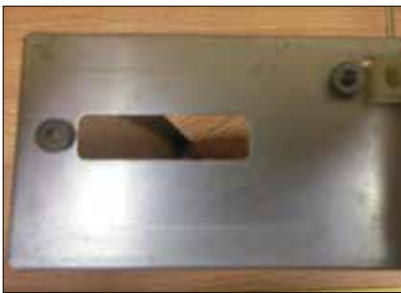
It was nice of Narco to leave this extra hole in the back of their transponder chassis for me to use as a cold air duct. Nice of them also to leave an extra press-nut for me to attach the temperature sensor.
