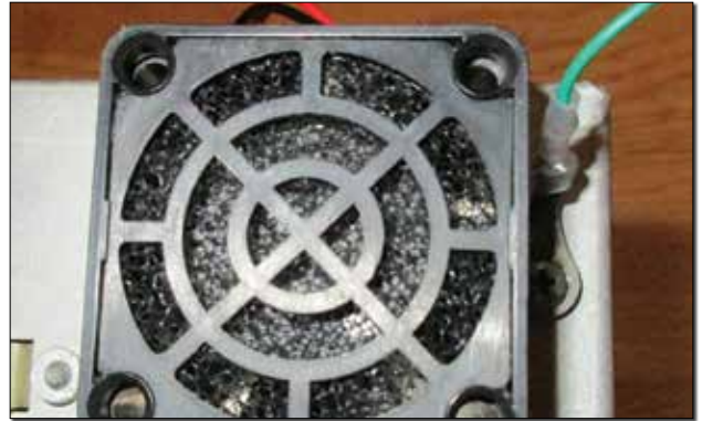
(Above) A diode temperature sensor mounted to a #4 solder lug for heat transfer. (Right) The fan mounted to the rear of the transponder case with the diode temperature sensor bolted to the right. Note the heat shrink on the diode.
