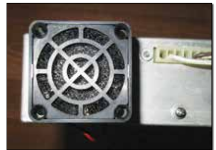
You can also get an air filter/finger guard for 40-millimeter fans from the same source.
