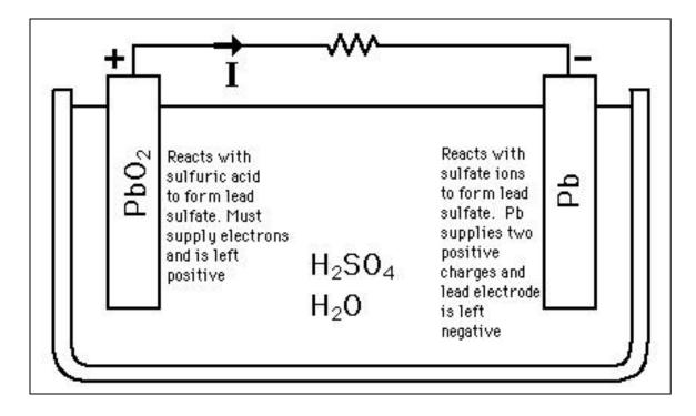
However, this particular chemistry is REVERSABLE. That is, you can draw current from the battery to power your circuit, but if you run electricity back in the reverse direction you can recharge the battery. We call these types of rechargeable batteries *SECONDARY CELLS*. The battery in your automobile is this lead-acid type of battery. You can use the battery to power a motor to start the car. Once started, your alternator runs current back through the battery to recharge it.
