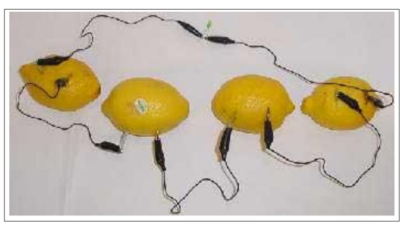
Fortunately, we have our choice of metals and electrolytes. In particular, copper and zinc are good metals to use (fairly high voltage and easy to come by), any citrus juice, vinegar (acetic acid), or a potato will work just fine. Copper can be obtained from copper wire (household romex cable, copper hookup wire, etc.), zinc can be obtained from any "galvanized" (zinc plated) metal such as galvanized steel, galvanized nails, etc.
