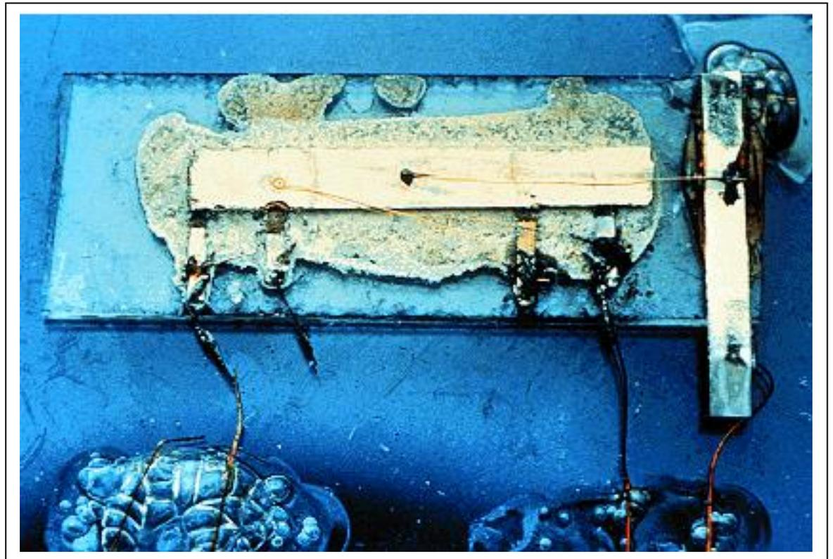
A little more work later with this newfangled silicon stuff and now we have entered the world of integrated circuits that really do the work. This photo of one of the first silicon integrated circuits shows a relatively clumsy design layout but in the late 1950s, it was state of the art.
