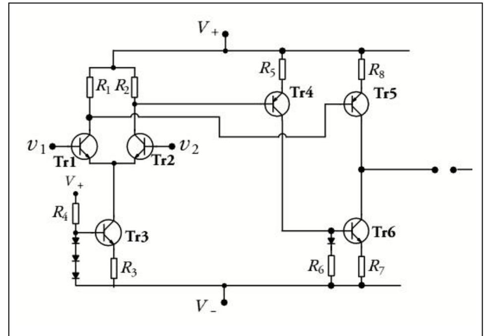
Almost. If there is a difference between the base-emitter diode voltages of Tr1 and Tr2, then it will appear to the output as though there is the same difference between  $v_1$  and  $v_2$ , and this diode difference voltage will be amplified right along with the signal difference. How do we get a difference of diode voltages? Heat up Tr1 and cool down Tr2 and just watch the output go nuts. (Go nuts, that's a technical term, you'll get used to it.)
