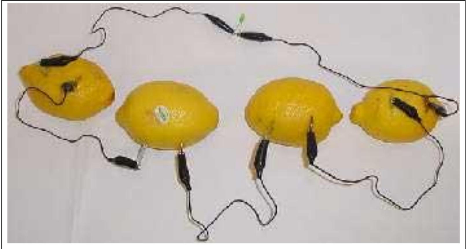
Fortunately, we have our choice of metals and electrolytes. In particular, copper and zinc are good metals to use (fairly high voltage and easy to come by), any citrus juice, vinegar (acetic acid), or a potato will work just fine. Copper can be obtained from copper wire (household romex cable, copper hookup wire, etc.), zinc can be obtained from any "galvanized" (zinc plated) metal such as galvanized steel, galvanized nails, etc.
