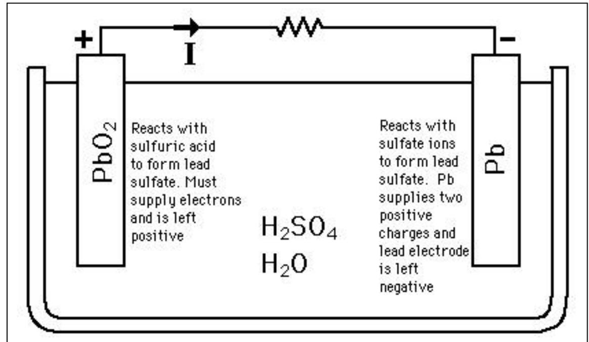
However, this particular chemistry is REVERSABLE. That is, you can draw current from the battery to power your circuit, but if you run electricity back in the reverse direction you can recharge the battery. We call these types of rechargeable batteries **SECONDARY CELLS**. The battery in your automobile is this lead-acid type of battery. You can use the battery to power a motor to start the car. Once started, your alternator runs current back through the battery to recharge it.
