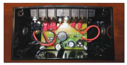
The PC board is "populated" with the circuit components, soldered together and put into the regulator chassis.
