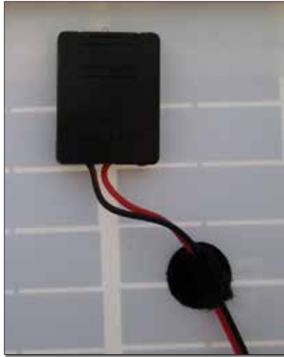
The box that keeps the wiring to the array itself enclosed (left). The controller hooked up, mounted to the hangar wall and ready for charging the aircraft battery (right).
