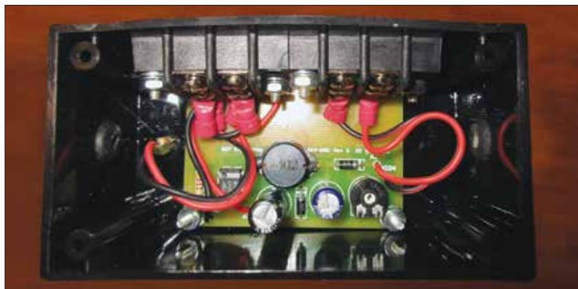
The PC board is “populated” with the circuit components, soldered together and put into the regulator chassis.
